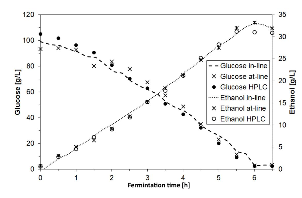
Monitoring of glucose and ethanol concentration in an aerobic batch fermentation of Saccharomyces cerevisiae. Comparison of in-line and atline Raman measurements as well as external HPLC reference analytics.
